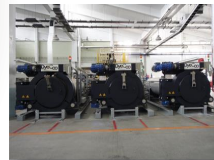
DyeCoo Supercritical CO 2 Water-Free Dyeing Machine
