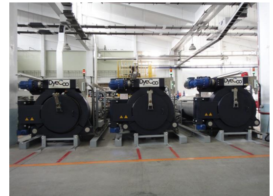
DyeCoo, super critical CO 2 fluid dyeing equipment
